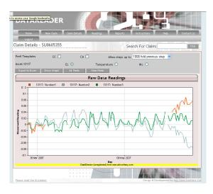
DataREADER interprets data from the new range of sensors using telemetry. This application retrieves data from the suppliers web site, graphs it and interprets it plus produces a report with just a few keystrokes by the user.
